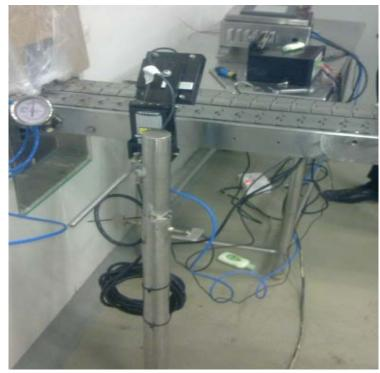
Deployed 160mm from its target, an P4-OMNI with 12mm C-Mount lens inspects for the location and presence of date and lot code and 2D-Code Reading on high speed Conveyor.
